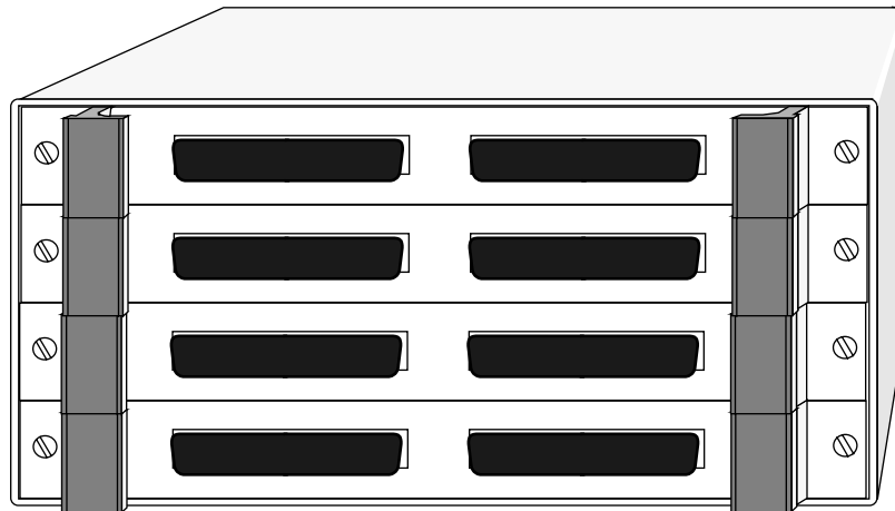
Figure 1. ENCL-4 Enclosure with Four EXP-1800s Installed
